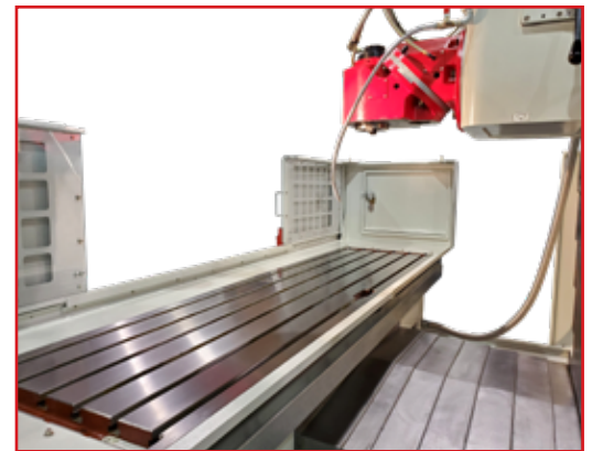
STEEL TELESCOPIC GUARD TO PROTECT BOX WAYS
